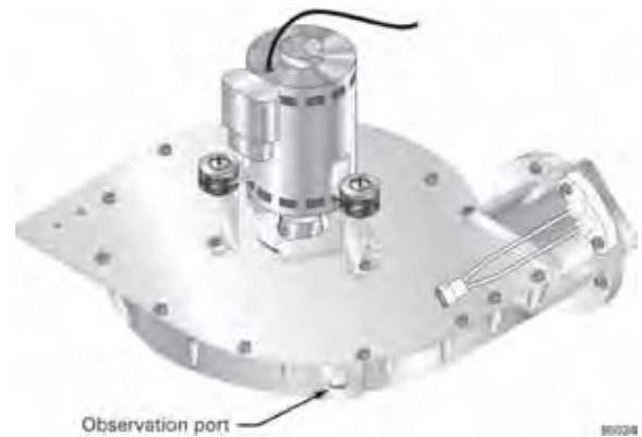
Figure 78 Igniter observation port in blower
