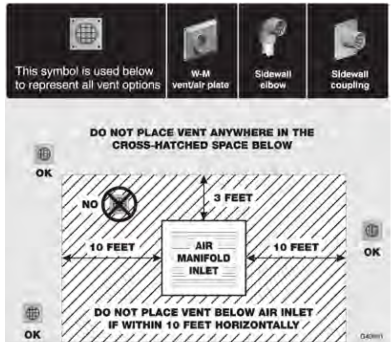
Figure 38 Maintain clearances and placement between the air manifold inlet and any appliance vent as shown below
