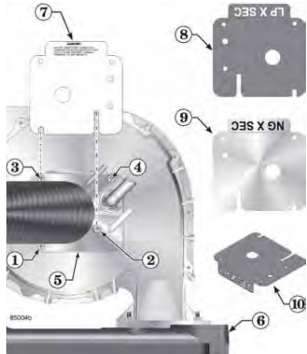
Figure 6 Follow instructions to check or replace gas orifice plate (“X” = boiler size)
