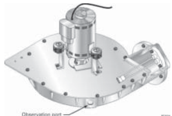
Figure 29 Igniter observation port in blower
